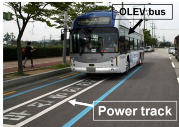
Figure 3: OLEV track, South Korea [24]. The OLEV bus drives on a power track that transmits electric flux during the drive. The cyan lines represent the optimal travel route that promises optimal energy transfer and charge. The receiver coils are mounted below the chassis of the bus, which receives the transmitted energy from the road and transfers it to the on-board battery.
