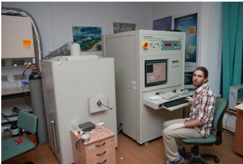
FIG. 3: CRESTEC BABLE 9000 high resolution electron beam lithography system (2 nanometer spot sized beam) at Bar-Ilan institute of Nanotechnology and advanced materials
