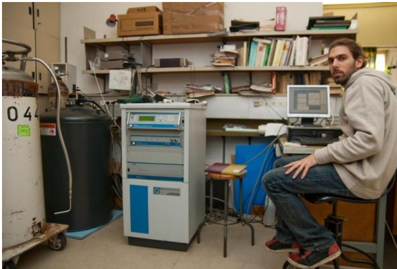
FIG. 4: Quantum Design Physical Property Measurement System (PPMS) installed at the Bar-Ilan Institute of Nanotechnology and Advanced Materials
