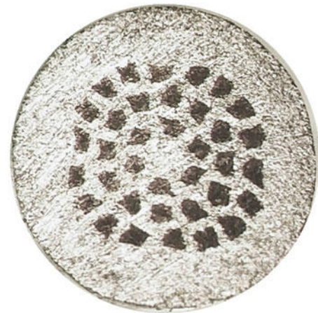
Fig. 3. Image of the cross-section of a 1.3 mm diameter, 36 filamentary \text{MgB}_2 wire with a Monel outer sheath.
