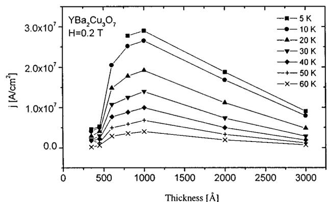
FIG. 3. Persistent current plotted vs thickness, at 0.2 T applied field, for various temperatures, between 5 K and 60 K. Lines are guide for the eye.
