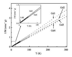
Fig. 1. Temperature dependence of the inverse of the paramagnetic part of the reciprocal magnetisation measured in the magnetic field of 0.2 T. The inset shows low-temperature data for the Gd2 and Gd4 glasses.
