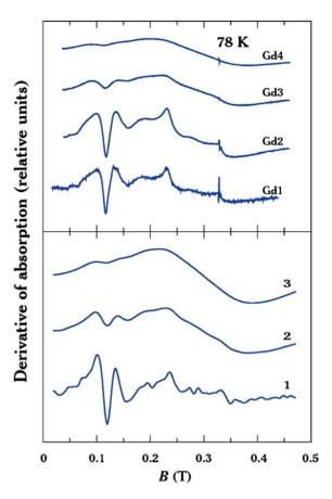
Fig. 2. Top: experimental EPR spectra. Bottom: computergenerated spectra assuming 100% of isolated ions (1), 70% isolated and 30% clustered ions (2) and 30% isolated and 70% clustered ions (3). The intrinsic lineshape for the isolated ions is Gaussian, with the linewidth  $\Delta_{\rm B} = 5$ , 10 and 15 mT for the (1), (2) and (3) curves, respectively. The clusters are described by a Gaussian lineshape with  $g_{\rm eff} = 2.25$  and  $\Delta_{\rm B} = 95$  mT.
