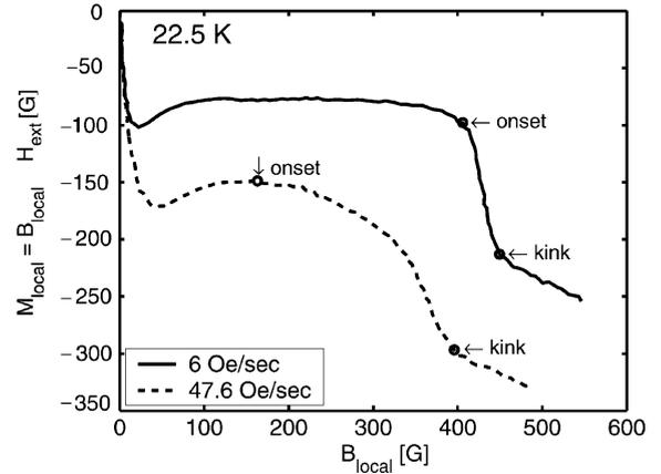
Fig. 2. Local magnetization vs. local induction at  $T = 22.5$  K, for sweep rates 47.6 Oe/s (dashed curve) and 6 Oe/s (solid curve). Curves were measured at  $x = -410 \mu\text{m}$  indicated by the vertical line in Fig. 1.
