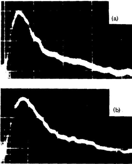
FIG. 2. (a) ir laser signal (as detected by a photon drag detector EL-OP Type 5413), and (b) the PE response in a SBN sample P-3 in case  $\tau_e \ll \mathcal{G}$ . Large division is 200 nsec horizontally and 1 mV vertically. Peak incident power on sample is 0.6 W.
