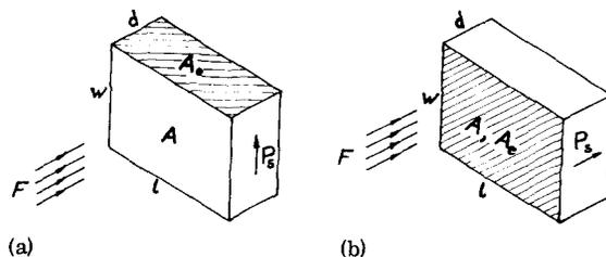
FIG. 1. Geometry of (a) edge- and (b) face-electroded pyroelectric samples.  $F$  is the radiation flux and  $P_s$  is the spontaneous polarization vector.
