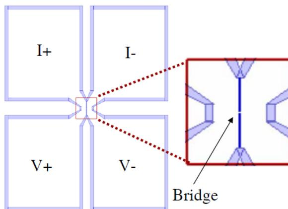
Figure 1. (Color on line) YBCO bridge and pads pattern. The blue color indicates the exposed areas which were removed after ion milling. The residue (white) shows the 4-peds connected to the bridge. The right panel zooms on the bridge area.
