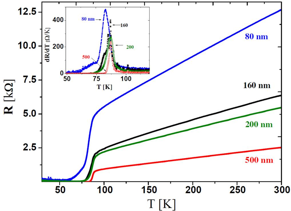
**Figure 2.** (Color on line). Temperature dependence of the zero-field resistance of 80, 160, 200 and 500 nm YBCO bridges (blue, black, green and red lines, respectively), measured with bias current of 5  $\mu$ A. The bridges are 700 nm long and 10 nm thick. Inset: Temperature derivative of the resistance for the four bridges.
