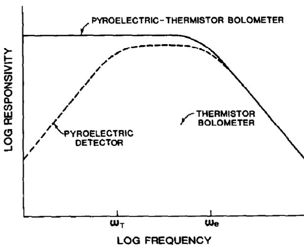
Fig. 1. A log-log plot of the frequency response of a thermistor bolometer, pyroelectric detector and tuned pyroelectric-thermistor bolometer.
