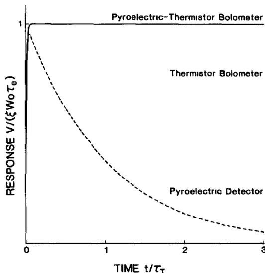
Fig 3 Responses of a thermistor bolometer, a pyroelectric detector and a tuned pyroelectric-thermistor bolometer to a step function
