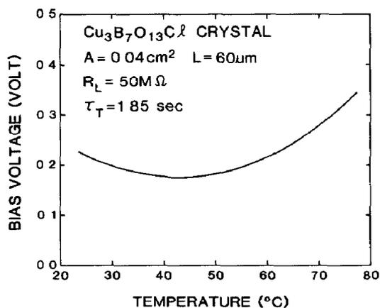
Fig 6 Temperature dependence of the bias voltage required for a uniform frequency response in a  $\text{Cu}_3\text{B}_7\text{O}_{13}\text{Cl}$  PTB
