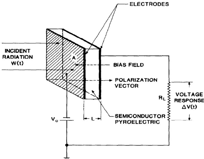
Fig. 2 A pyroelectric thermistor bolometer
