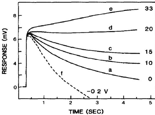
Fig 5 Oscillograms of the output voltage of a  $\text{Cu}_3\text{B}_7\text{O}_{13}\text{Cl}$  PTB in response to a step illumination for different bias voltages
