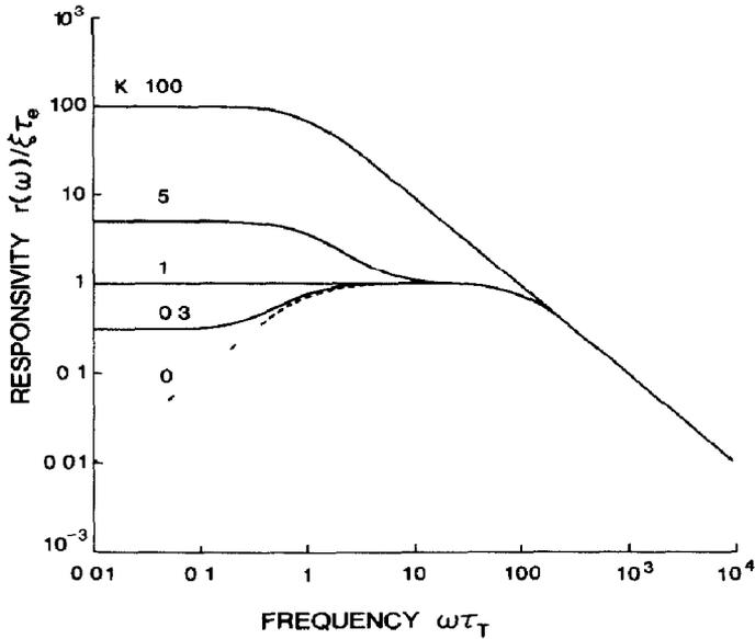
Fig 4 Frequency response of a pyroelectric-thermistor bolometer for  $\theta = 0.01$  and different values of  $k$
