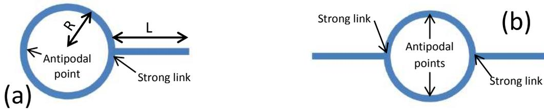
**Figure 6.** (a) An illustration of a superconducting ‘lasso’: a ring with radius  $R$  attached with an arm with length of  $L$ . (b) An illustration of a superconducting ring with two arms.
