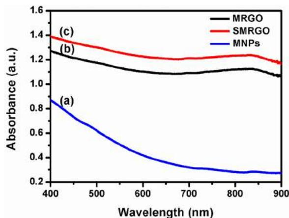
**Figure 5.** UV-vis-NIR spectra of (a) MNPs, (b) SMRGO, and (c) MRGO.
