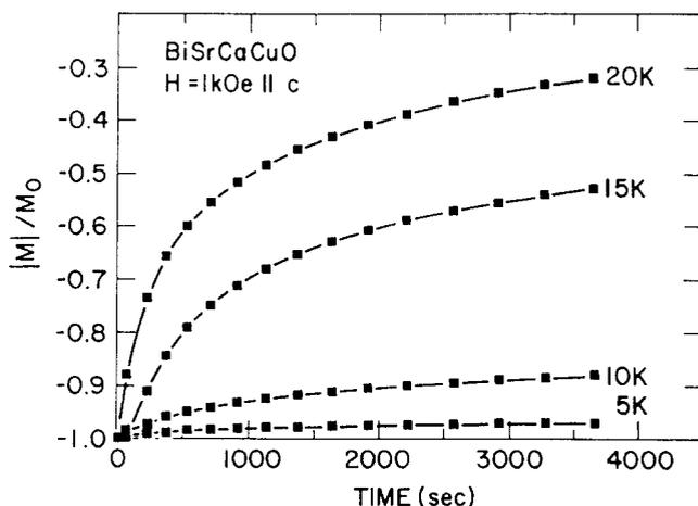
**Figure 3** Decay of the normalized magnetization as a function of time for a BiSrCaCuO crystal. The field  $H = 1$  kOe, parallel to  $c$ , is applied after cooling the sample in zero field
