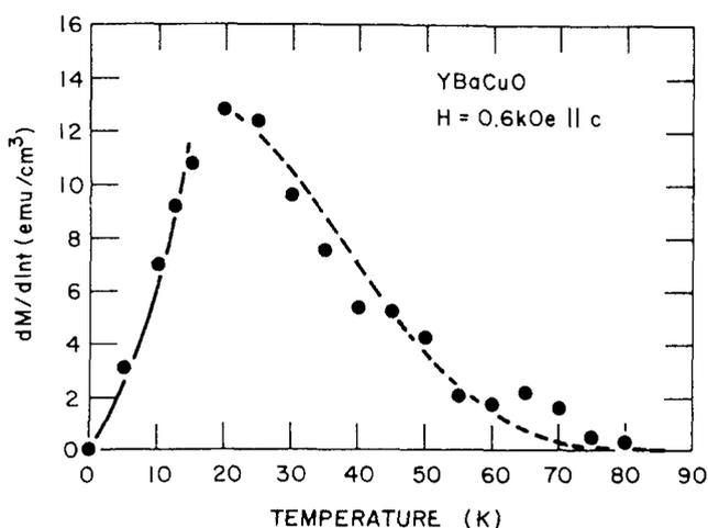
**Figure 2** Relaxation rate of the zero-field-cooled magnetization as a function of temperature for field 0.6 kOe parallel to the orthorhombic  $c$ -axis of a YBaCuO crystal. Solid line is a fit to Equation 1 with  $U_0(0) = 0.015 \text{ eV}$ . Broken line is a guide for the eye for  $H > H^*(T)$  (from Reference 4)
