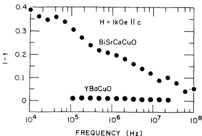
Figure 5 Frequency dependence of the irreversibility reduced temperature  $1 - T_{irr}/T_c$  of a twinned YBaCuO crystal and a BiSrCaCuO crystal determined by a.c. susceptibility for an applied field of 1 kOe applied along the  $c$  axis.
