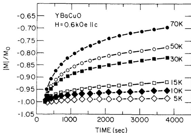
**Figure 1** Decay of the normalized magnetization as a function of time for a YBaCuO crystal. The field  $H = 0.6 \text{ kOe}$ , parallel to  $c$ , is applied after cooling the sample in zero field (from Reference 4)
