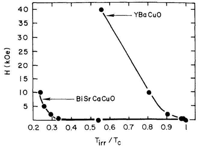
Figure 6 Field dependence of the reduced temperature  $1 - T_{irr}/T_c$  of a twinned YBaCuO crystal and a BiSrCaCuO crystal determined by standard zfc/fc measurements with the field applied along the  $c$  axis
