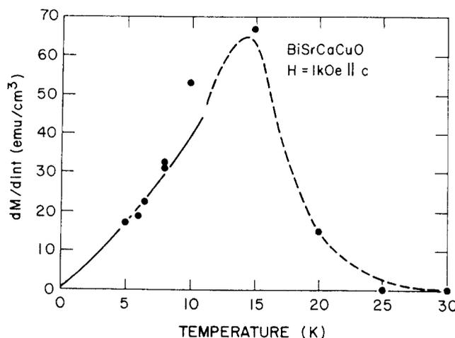
**Figure 4** Relaxation rate of the zero-field-cooled magnetization as a function of temperature for field 1 kOe parallel to the orthorhombic  $c$ -axis of a BiSrCaCuO crystal. Solid line is a fit to Equation 1 with  $U_0(0) = 8 \times 10^{-4}$  eV. Broken line is a guide to the eye
