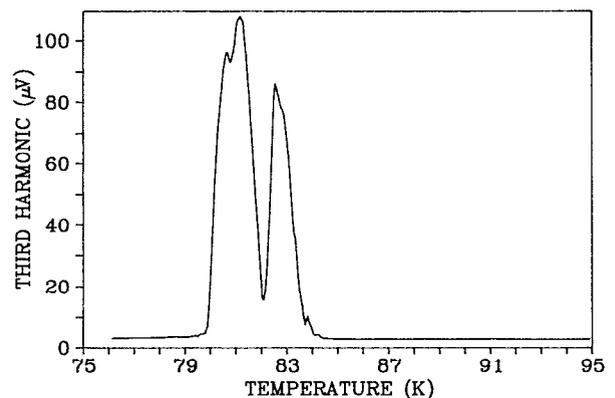
FIG. 3. Measured third harmonic susceptibility in Y-Ba-Cu-O thin-film sample prepared by activated reactive evaporation method.
