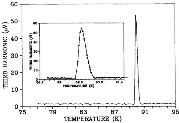
FIG. 4. Measured third harmonic susceptibility in Y-Ba-Cu-O thin-film sample prepared by laser ablation technique.
