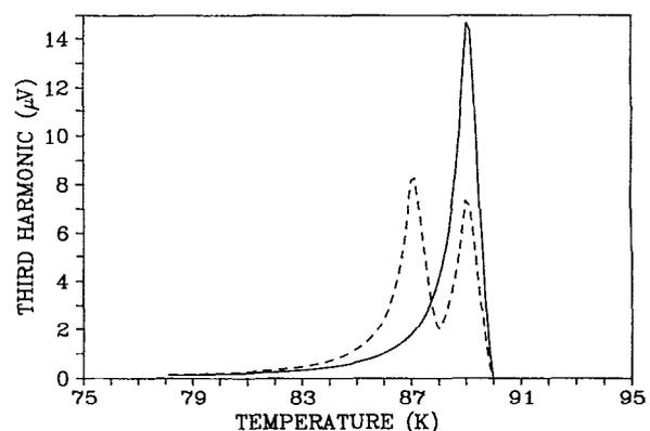
FIG. 1. Calculated third harmonic susceptibility in single phase (solid line) and two-phase (dashed line) superconducting samples.
