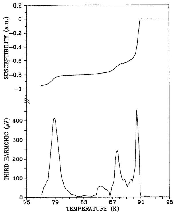
FIG. 2. Measured linear (upper curve) and third harmonic (lower curve) susceptibilities in Y-Ba-Cu-O thin-film sample prepared by electron-beam evaporation technique.
