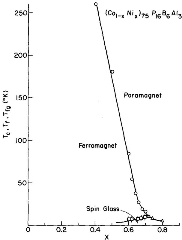
Fig. 2 Magnetic phase diagram for  $(\text{Co}_{1-x}\text{Ni}_x)_{75}\text{P}_{16}\text{B}_6\text{Al}_3$ .
