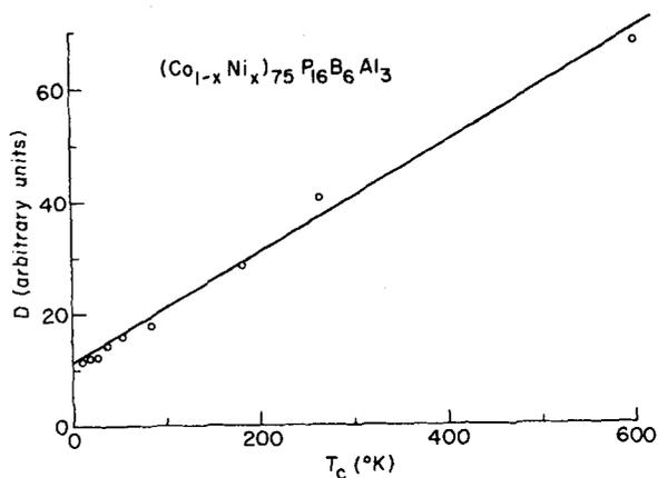
Fig. 5. Stiffness constant  $D$  as a function of Curie temperature  $T_c$ .
