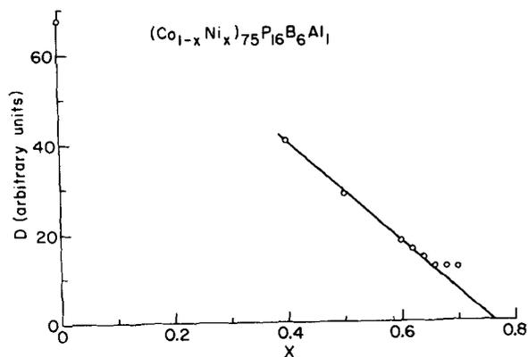
Fig. 4. Stiffness constant  $D$  as a function of Ni concentration  $x$ .
