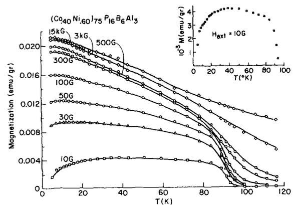
Fig. 1 Temperature dependence of the magnetization for  $(\text{Co}_{.40}\text{Ni}_{.60})_{75}\text{P}_{16}\text{B}_6\text{Al}_3$  for different applied fields. Insert shows  $M(H,T)$  for  $H_{ext} = 10\text{G}$ .
