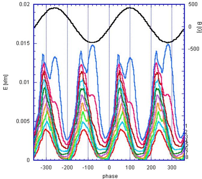
Fig. 3.  $E(t)$  graphs of Bi-2223 tape exposed to AC magnetic field at 23 Hz, 400 G rms.  $E(t)$  curves are shown for DC currents of 140 A(1), 130 A(2), 120 A(3), 110 A(4), 100 A(5), 90 A(6), 80 A(7), 70 A(8).
