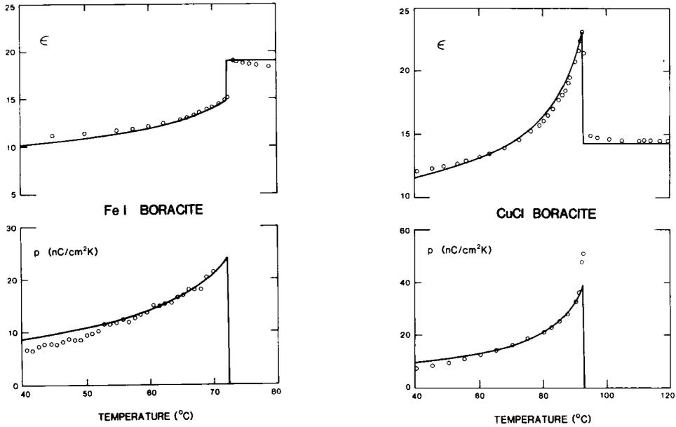
FIGURES 1,2,3 Theoretical curves fitted to the measured values of the dielectric constant and pyroelectric coefficient of FeI, CuCl and MnI boracites. The parameter values used in the fits are given in Table 1.
